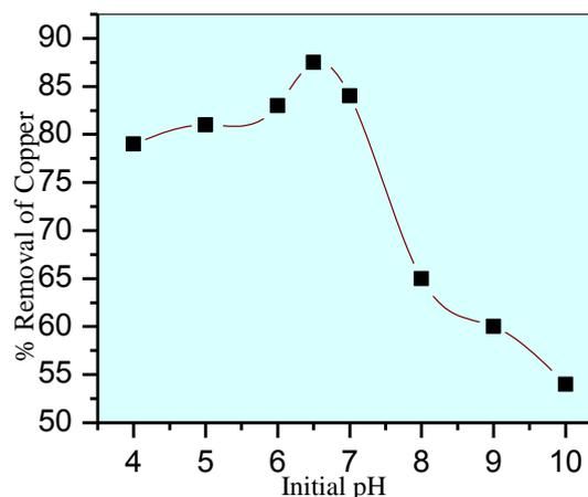
Fig:3- Effect of Initial pH on the removal of Cu(II) Ion
