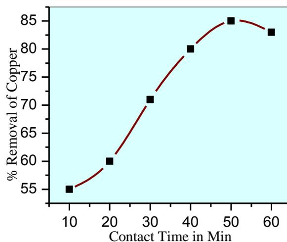
Fig:1- Effect of Contact Time on the Removal of Cu(II) Ion [Cu]=50 mg/L; Temperature 30°C; Adsorbent dose=25mg/50ml
