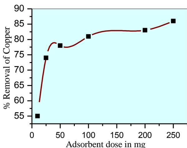
Fig:2- Effect of Adsorbent dose on the removal of Cu(II) Ion
