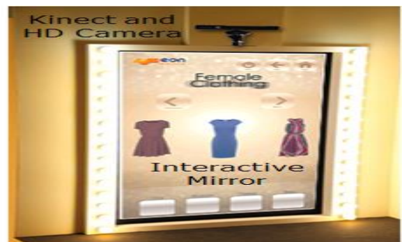
Figure 6. The front view of the Interactive Mirror with Kinect and HD camera placed on top.
