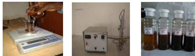
Figure 3.2: Weighing and Probe sonication of CuO-Engine oils.
