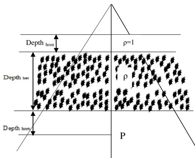
**Figure 1.** Schematic diagram showing a water equivalent phantom ( $\rho=1$ ) containing an inhomogeneity of electron density ( $\rho$ ) relative to water. P is the point of dose calculation.
