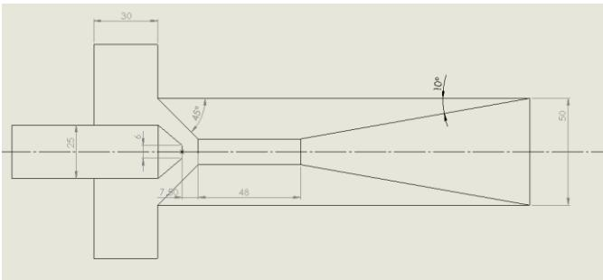
**Figure 3.** mixing nozzle angle with  $45^{\circ}$
