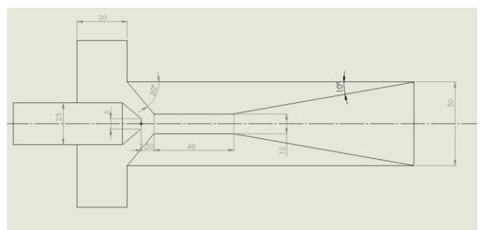
**Figure 2.** mixing nozzle angle with  $50^0$
