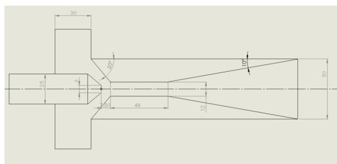
**Figure 2.** mixing nozzle angle with  $50^\circ$
