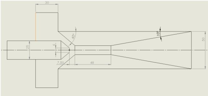
**Figure 4.** mixing nozzle angle with  $40^{\circ}$
