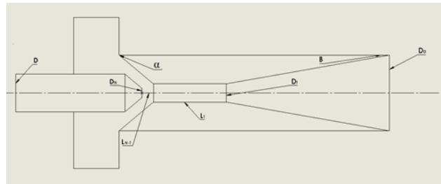
**Figure 1.** Schematic View of Jet Pump.
