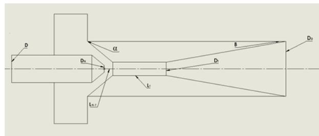
**Figure 1.** Schematic View of Jet Pump.
