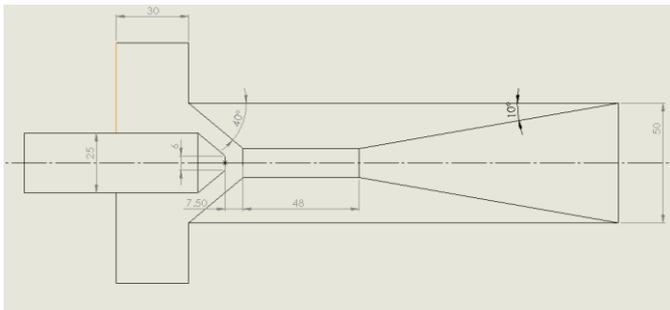
**Figure 4.** mixing nozzle angle with 40°
