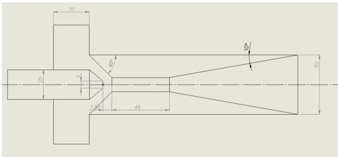
**Figure 3.** mixing nozzle angle with 45°
