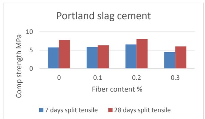
**Effect of Recron fiber on Splitting Tensile Strength using slag:**
