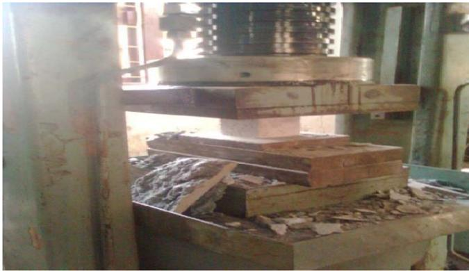
Figure 3. Compressive test on cube
