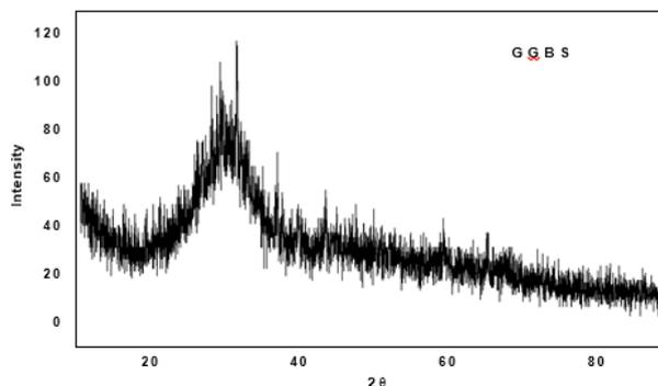
**Figure 1.** X-Ray Diffraction test of GGBS
