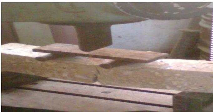
Figure 5. Flexural test on Beam
