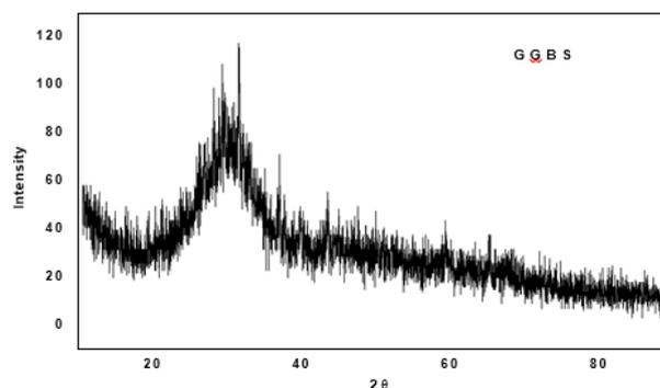
**Figure 1.** X-Ray Diffraction test of GGBS
