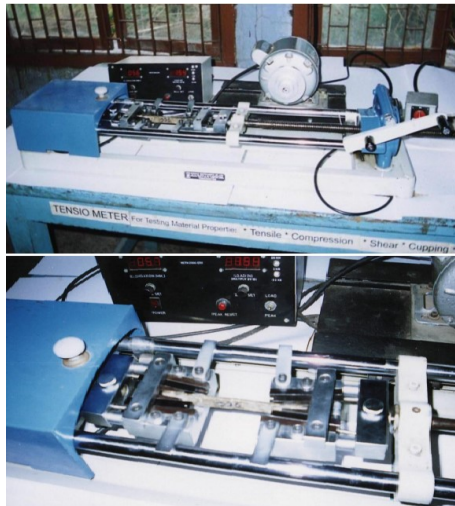
Figure 6. Strength measuring equipment Tensiometer
