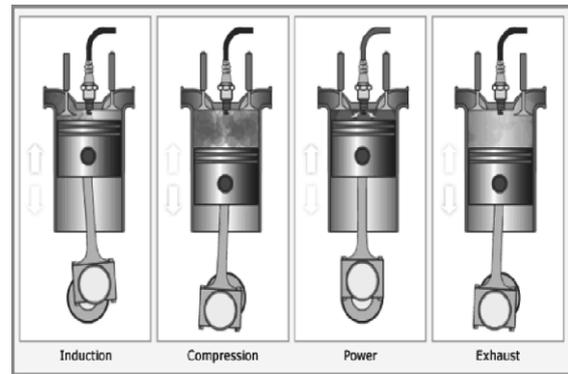
An internal combustion engine is defined as an engine in which the chemical energy of the fuel is released inside the engine and used directly for mechanical work, as opposed to an external combustion engine in which a separate combustor is used to burn the fuel.
