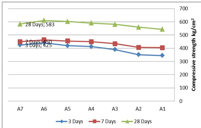
According to Table 4, Compressive strength in all mixes increased with time and with increases in activator ratio up to sample A6 then the compressive strength decreases with ratio increases. These behaviors are matched with above determinations in air and in oven.
