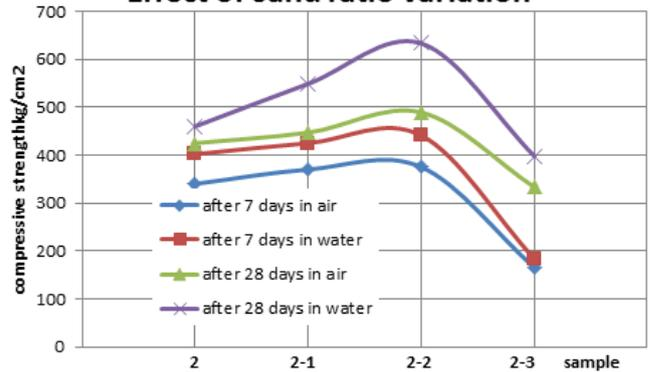
According to table 6 the best results obtained at 28 days that include sand ratio 0.5 of basalt weight in concrete and recording 653 kg/cm<sup>2</sup> in water curing. While in air the best result obtained at sand ratio 0.25 of basalt weight in concrete and recording 447 kg/cm<sup>2</sup> in water curing at 28 days in water curing.
