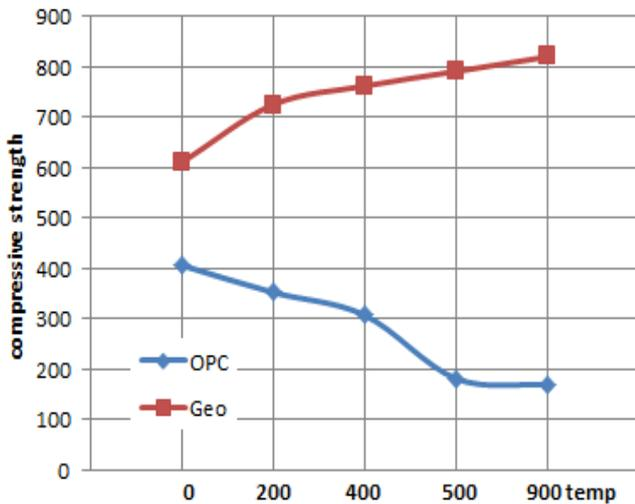
Table 8 shown sharply decreases in compressive strength of OPC with increasing in firing temperature. In case of new geopolymer cement the compressive strength increases up to 900 C<sup>0</sup> and recording 820 kg/cm<sup>2</sup>.
