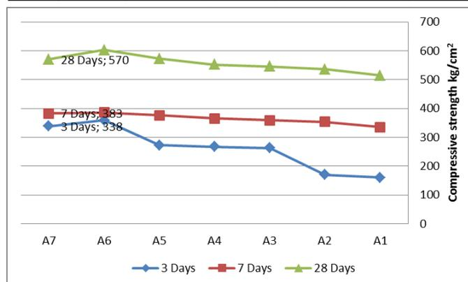
Table 2 shown increases in compressive strength of Geopolymers cement with time and this increases gets highly strength at sample A6 which included SiO<sub>2</sub>/NaO ration equal 5. And this behavior change with increasing of ratio as shown in sample A7.
