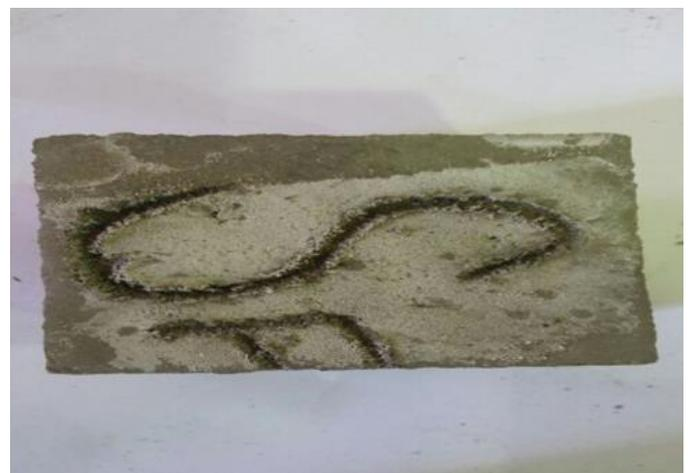
Figure 2. Variation in Geopolymers cement with firing at 900 C<sup>0</sup>
