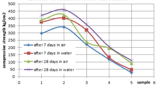
Table 5 shown best mix cement and coarse aggregate are obtained in **mix 2** which get compressive strength 425 kg/cm<sup>2</sup> in air setting and 460 kg/cm<sup>2</sup> in water curing after 28 days.
