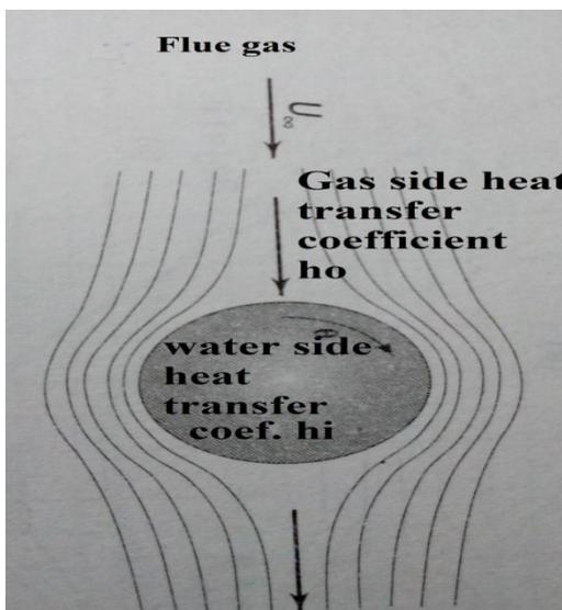
**Figure 4:** Flow over a circular cylinder
