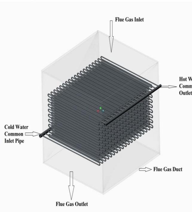
**Figure 7:** Designed 3D view of cross flow heat exchanger
