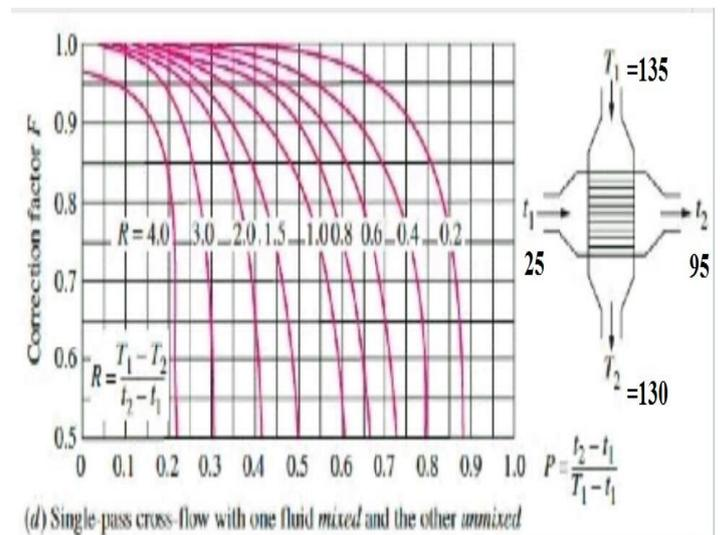
**Figure 5:** Correction factor calculation for cross flow heat exchanger
