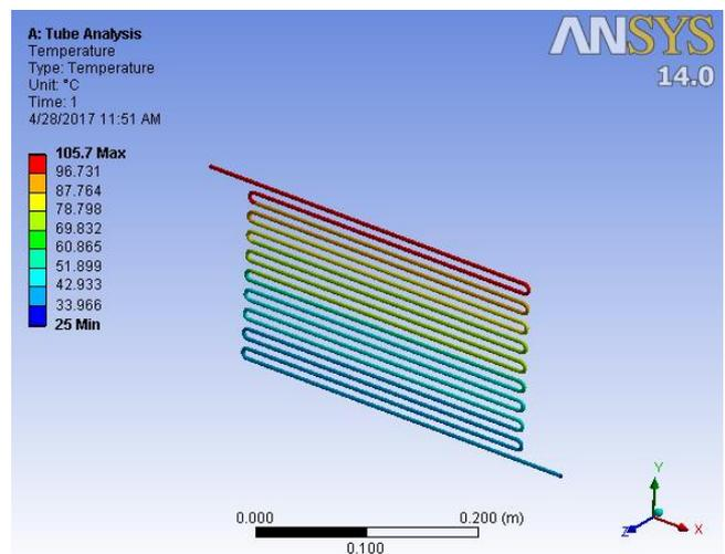
**Figure 10:** Temperature contour of inner walls of a column
