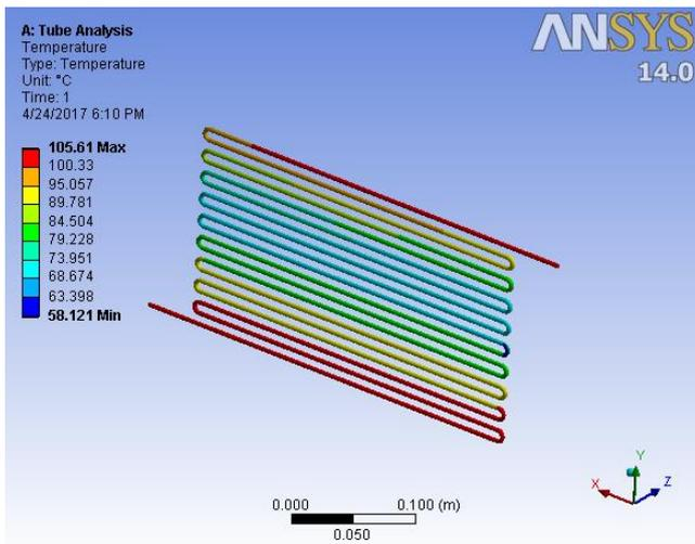
**Figure 11:** Temperature contour of outer walls of a column
