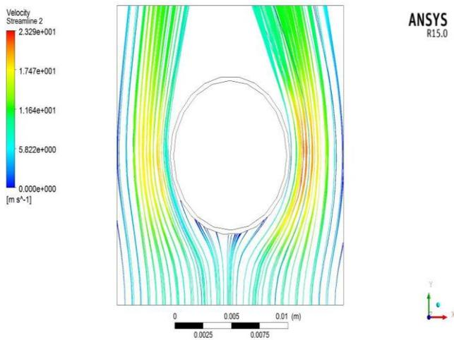
**Figure 8:** Velocity Streamline of Flue Gas
