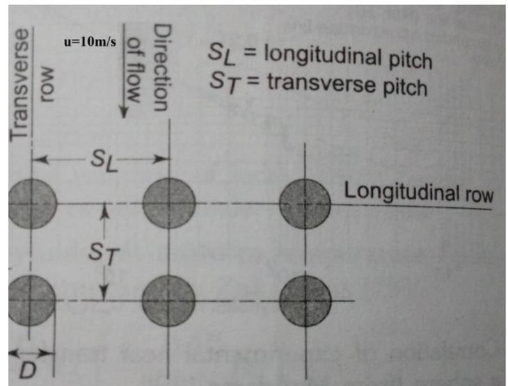
**Figure 3:** In-line tube arrangement in cross flow heat exchanger
