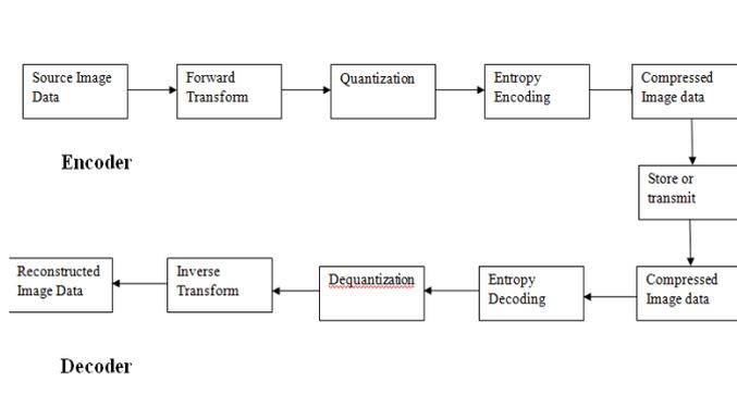
Figure 2. Basic Architecture of JPEG2000
