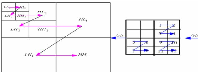
Figure 3.(a) The scanning sort of SPIHT algorithm and wavelet coefficients (b) the scanning sort of SPIHT algorithm in the same frequency band.
