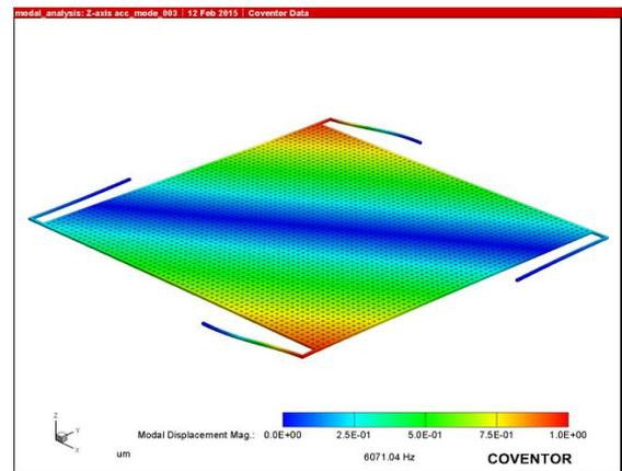
Figure: 3.3 Third resonant mode of the accelerometer
