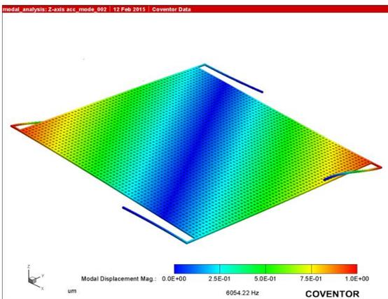
Figure: 3.2 Second resonant mode of the accelerometer
