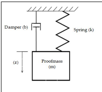
**Figure: 2** Dynamic model of out-of-plane accelerometer shown in equation (2),
