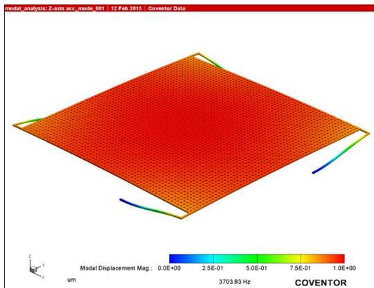
Figure: 3.1 First resonant mode of the accelerometer
