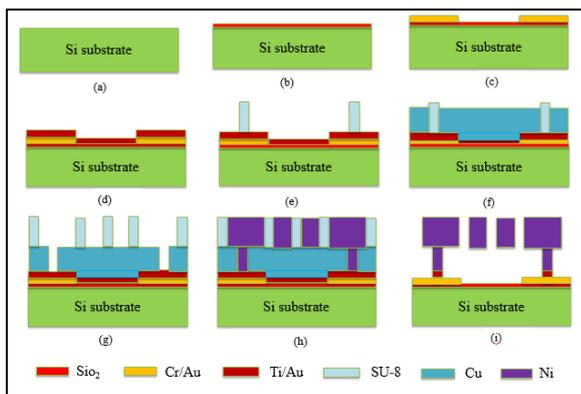
**Figure : 4** Fabrication methodology of Accelerometer fabrication process: (a) Silicon substrate (b) oxidation on substrate (c) formation of anchors and contact pads of gold in 1<sup>st</sup> lithography (d) sputtering of Au seed layer (e) coating of SU-8 using 2<sup>nd</sup> level mask (f) Electroplating of copper (g) coating of SU-8 using 3<sup>rd</sup> level mask (h) Electroplating of Nickel (i) Released structure after etching of SU-8, copper and Au seed layer.
