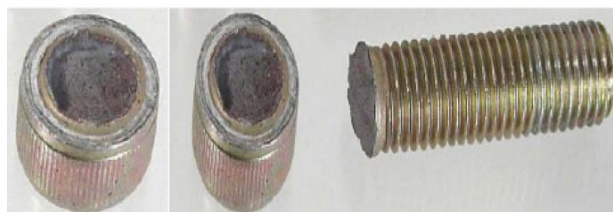
Figure 2: Typical Fastener Failure by Hydrogen Embrittlement [8]
