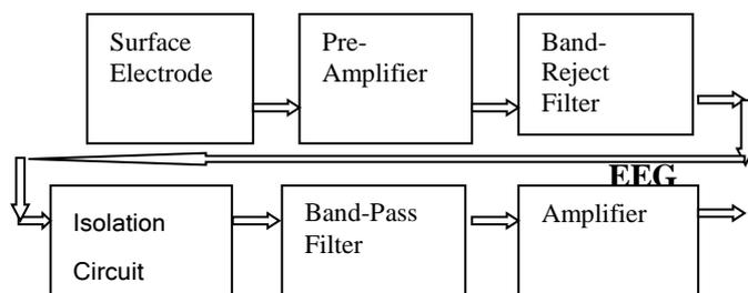
Figure 1 : Block diagram of EEG measurement Circuit.
