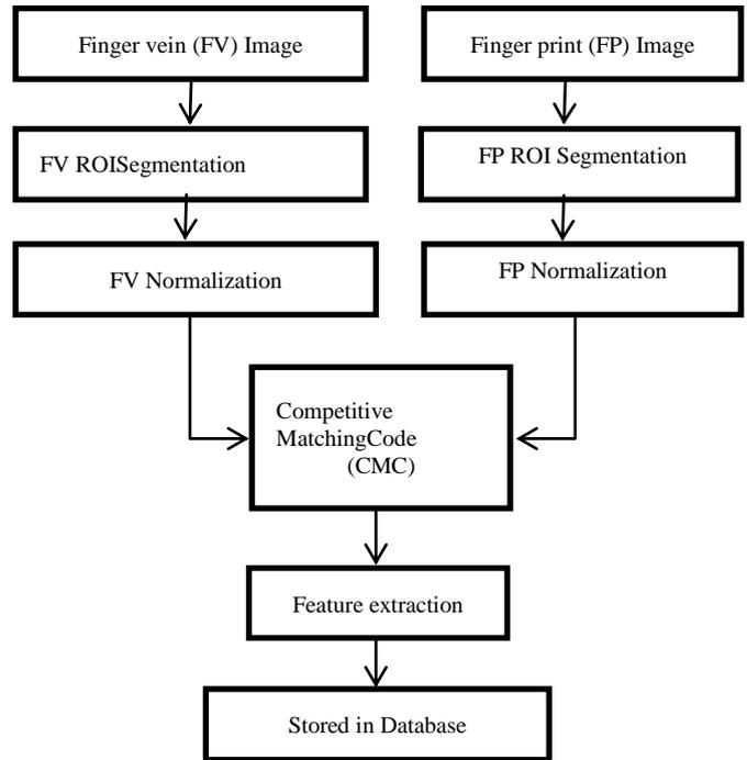
Figure 3: Proposed Verification frame work
