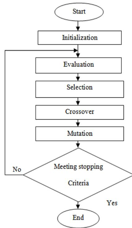
Figure 13. Flow chart of the genetic algorithm.
