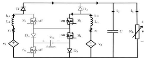
Figure 3. Condition State 2 ( $d_1T < t < d_2T$ )
