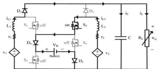
Figure 11. Condition State 3 ( $d_1 T < t < d_2 T$ )
