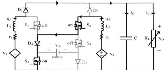
**Figure 7. Condition State 3 ( $d_1T < t < d_2T$ )**
