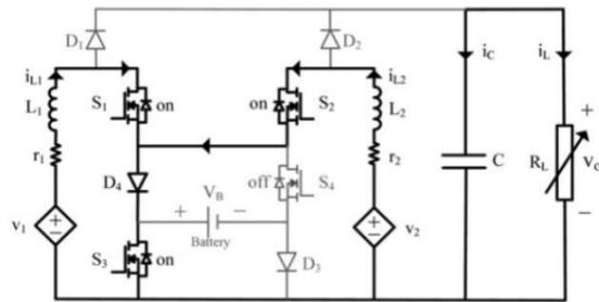
**Figure 6. Condition State 2 ( $d_4T < t < d_1T$ )**
