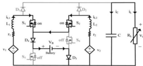
Figure 10. Condition State 2 ( $d_3 T < t < d_1 T$ )
