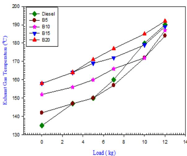
**Figure 9 :** Graph showing Exhaust Gas Temperature against different Loads (Kg) for pure diesel and combination of KOME blend
