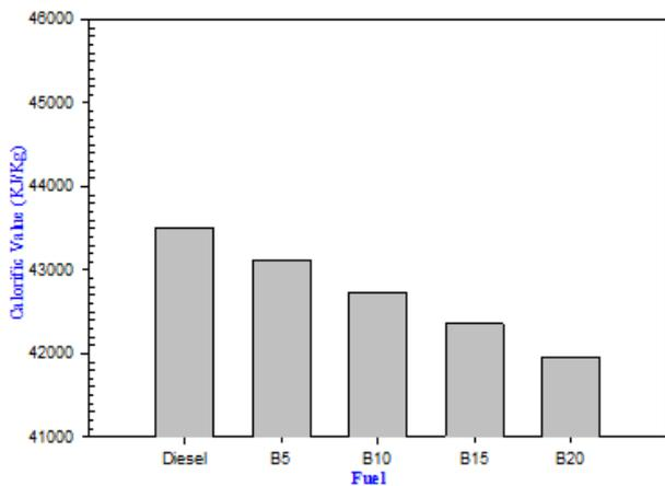
**Figure 1:** Calorific Values of Karanja Blend Fuels
