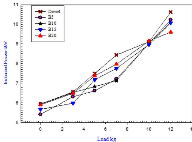
**Figure 4:** Graph showing Indicated Power (KW) against different Load (Kg) for pure diesel and combination of KOME blend
