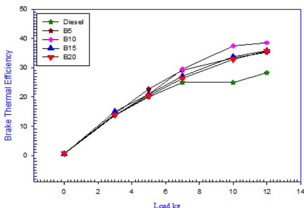
**Figure 6 :** Graph showing Brake Thermal Efficiency against different Loads (Kg) for pure diesel and combination of KOMBE blend
