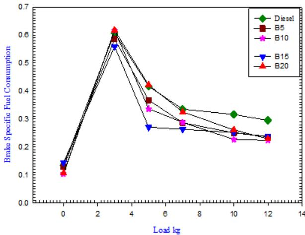
**Figure 8:** Graph showing Brake Specific Fuel Consumption against different Loads (Kg) for pure diesel and combination of KOME blend.
