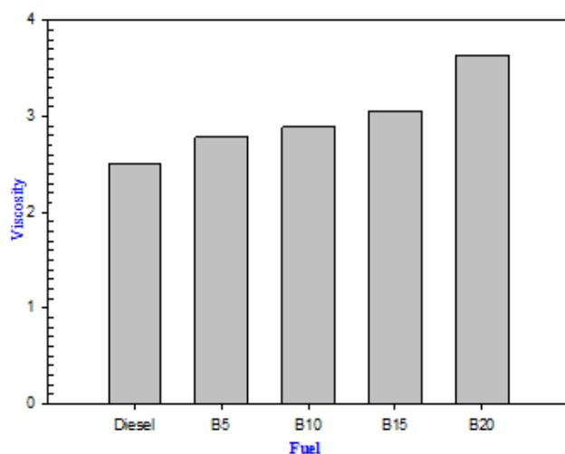
**Figure 2:** Viscosity of Diesel with Karanja Blends
