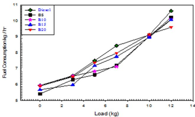
**Figure 5:** Graph showing Fuel Consumption (Kg/hr) against different Loads (Kg) for pure diesel and combination of KOMBE blend
