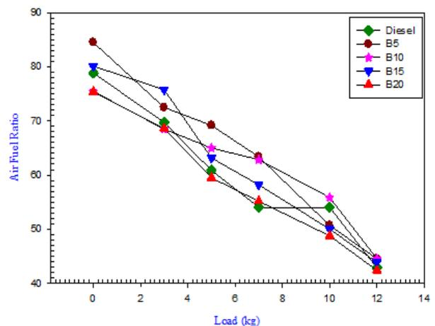
**Figure 7:** Graph showing Air Fuel Ratio against different Loads (Kg) for pure diesel and combination of KOMBE blend
