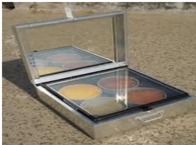
Figure 4: Schematic view of Box type solar cooker.
