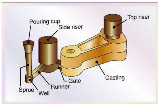
**Figure 3:** Parts of Typical Gating System
