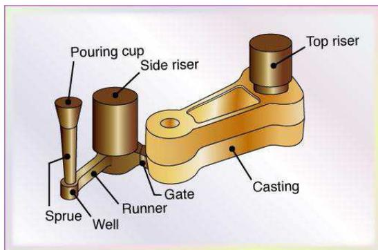
**Figure 3:** Parts of Typical Gating System
