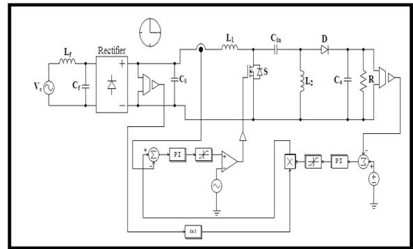
**Figure 5.** Circuit diagram for average current control with voltage follower approach for the proposed SEPIC converter
