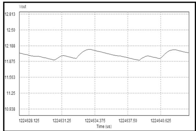
**Figure 6(b).** Simulation waveforms of output voltage and current for borderline control technique of the SEPIC converter
