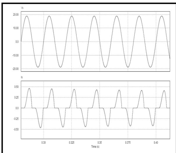
**Figure 3(a).** Simulation waveforms of input voltage and current of the SEPIC converter in open loop control
