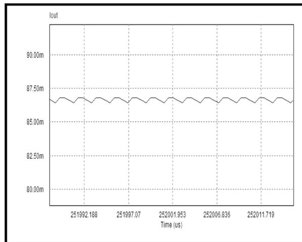
**Figure 3(b).** Simulation waveforms of output voltage and current of the SEPIC converter in open loop control
