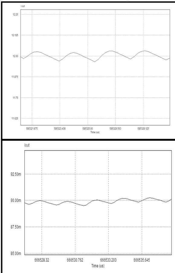
**Figure 4(b)** Simulation waveforms of output voltage and current of the SEPIC converter in voltage follower approach
