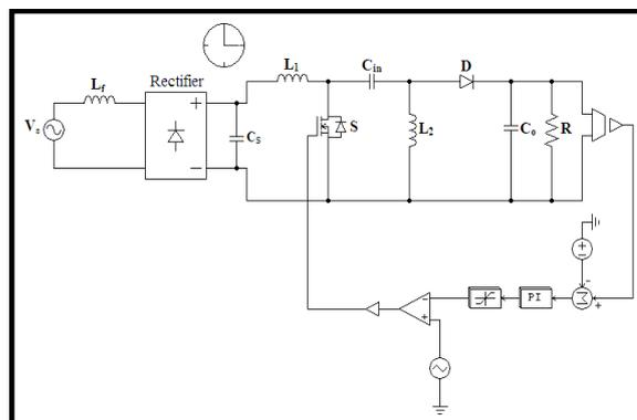
**Figure 4.** Circuit diagram for voltage follower approach of proposed SEPIC converter
