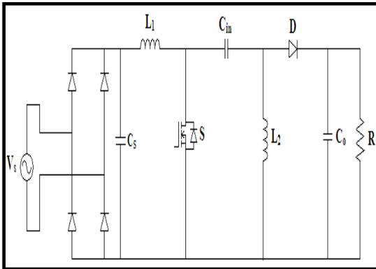
**Figure 2.** Circuit diagram of the proposed converter
