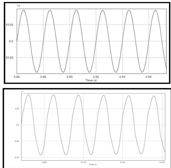
**Figure 5(a)** Simulation waveforms of input voltage and current for average current control with voltage follower approach of the SEPIC converter
