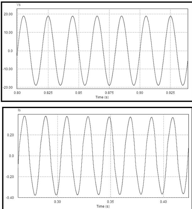
**Figure 6(a).** Simulation waveforms of input voltage and current for borderline control technique of the SEPIC converter
