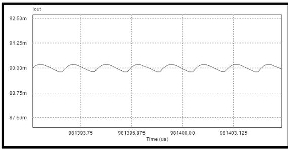
**Figure 5(b).** Simulation waveforms of output voltage and current for average current control with voltage follower approach of the SEPIC converter
