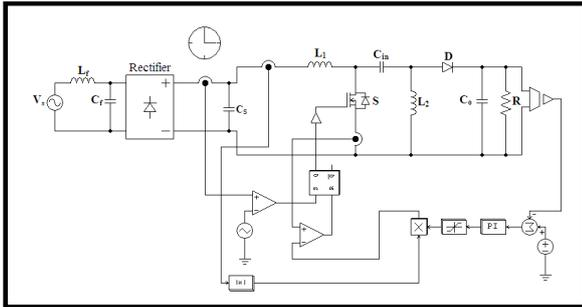
**Figure 6.** Circuit diagram of borderline control technique for proposed SEPIC converter
