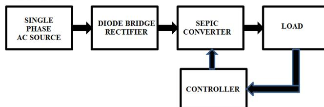
Figure 1: Block diagram of the proposed converter circuit
