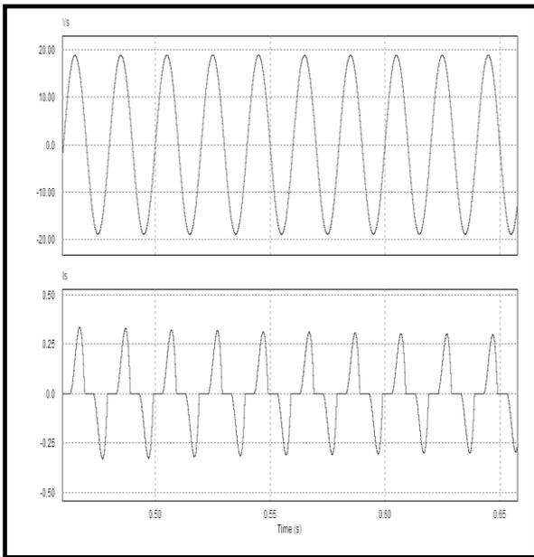
**Figure 4(a).** Simulation waveforms of input voltage and current of the SEPIC converter in voltage follower approach
