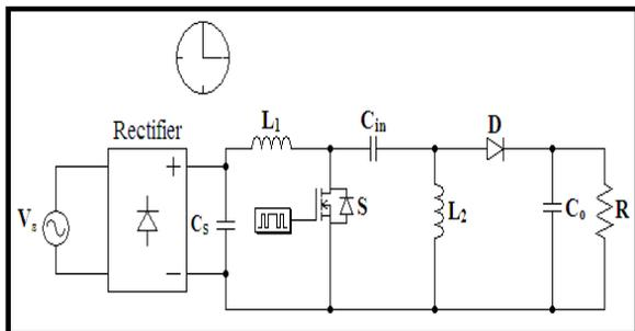
**Figure 3.** Circuit diagram for the open loop control of the proposed SEPIC converter
