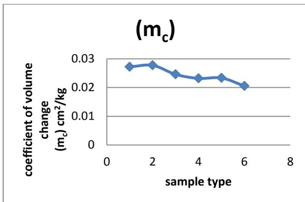
**Graph-7:** Variation of Coefficient of Volume Change for different % of GGBS and Jute Fibre
