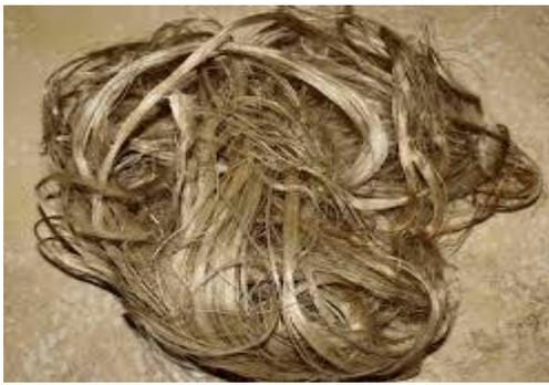
Figure 1. Jute Fibre
