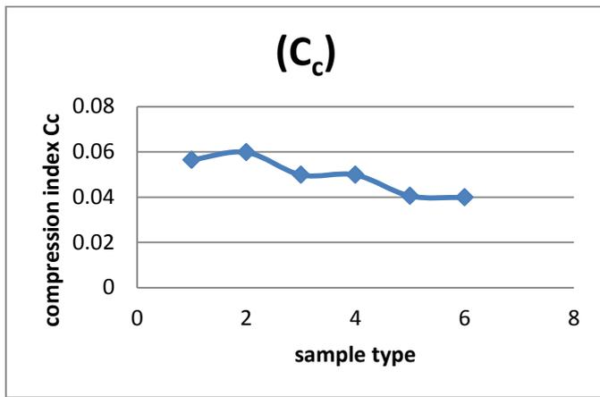
**Graph-6:** Variation of Compression Index for different % of GGBS and Jute Fibre
