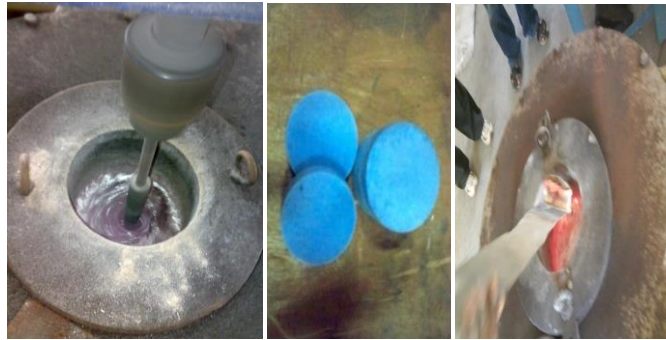
Fig. 5. Molten Metal, Fig. 6. degas tablet Fig. 7. Adding Metal, Degasifier reinforcment Materials
