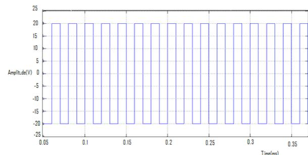
**Figure 8 :** Losing drive pulse fault
