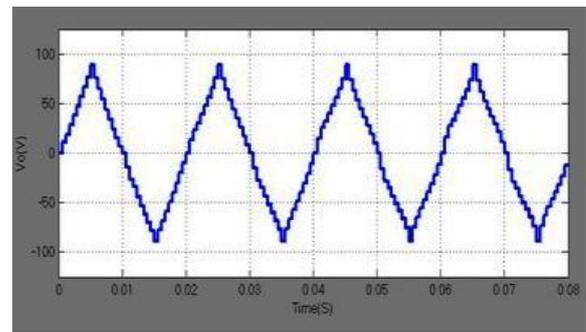
**Figure 5:** Normal 19 Level waveform
