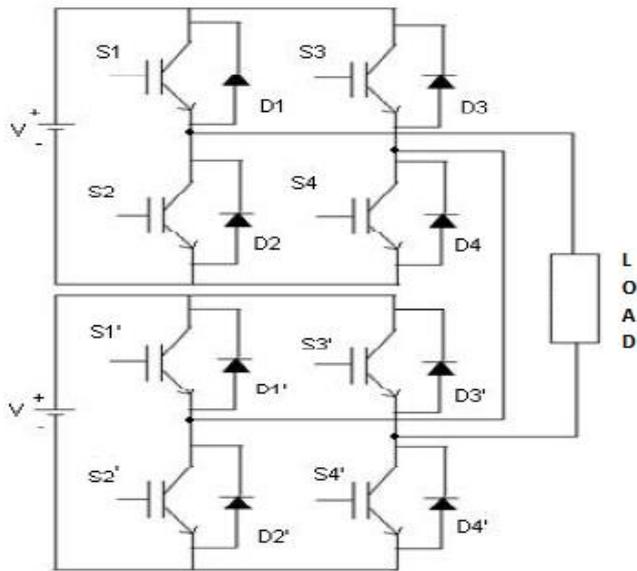
**Figure 1:** Five level Cascaded Multilevel Inverter
