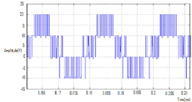
**Figure 6 :** open circuit fault
