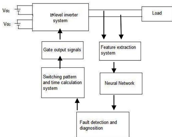
**Figure 3:** Structure of fault diagnostic system
