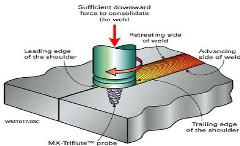
**Figure 2:** A Schematic Diagram Of Friction Stir Welding Process [7]
