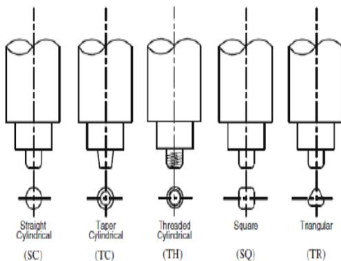
**Figure 2 :** Schematic diagram of the FSW tool. [7]
