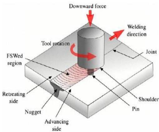
**Figure 1 :** Schematic diagram of friction stir welding process [6]
