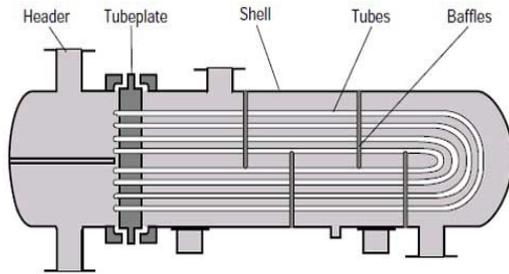
**Fig 1- U tube heat exchanger**
