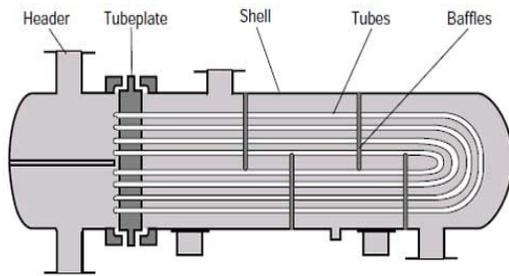
**Fig 1- U tube heat exchanger**
