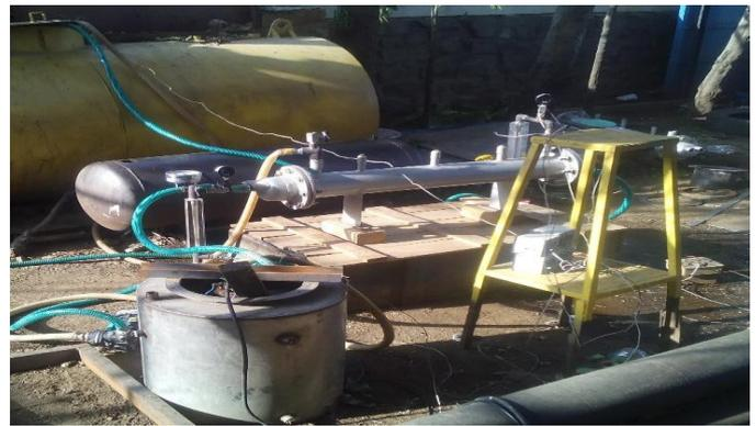
**Fig 3. Photo of Experimental set up of STHX**
