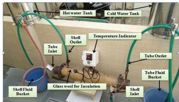
Fig 4. Photo of Experimental set up of STHX
