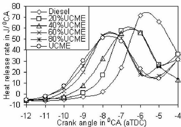
Figure 6. Comparison of rate of heat release
