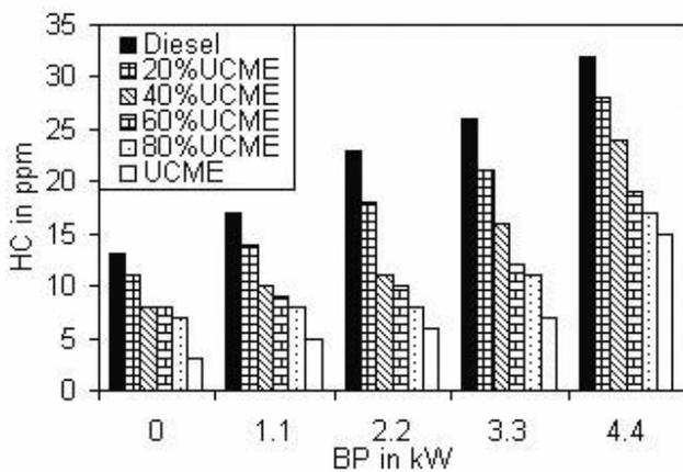
**Figure 12.** Comparison of hydrocarbon emissions
