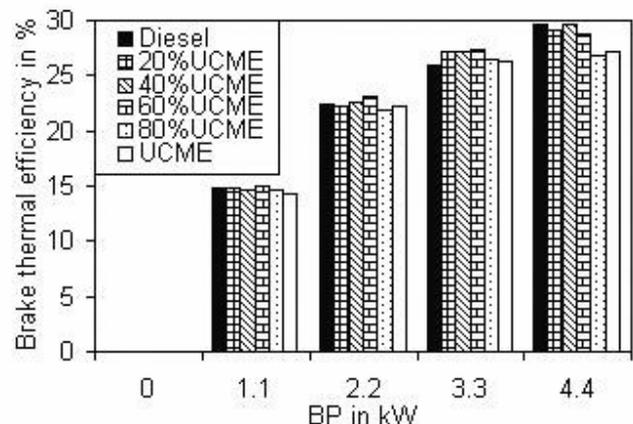
Figure 8. Comparison of brake thermal efficiency
