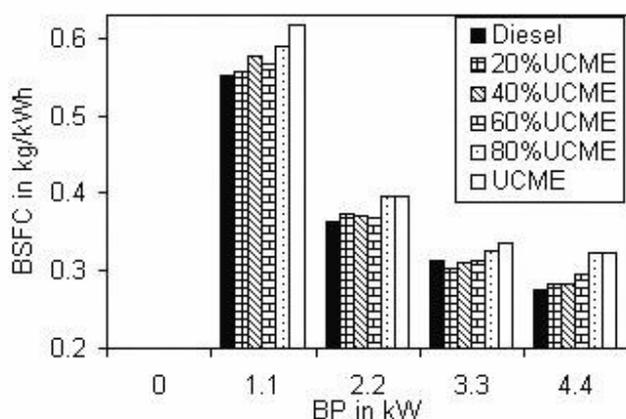
Figure 7. Comparison of brake Specific fuel consumption
