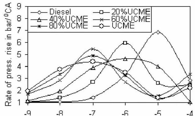
**Figure 4.** Comparison of Rate of Pressure Rise
