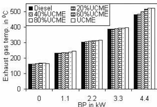
**Figure 10.** Comparison of exhaust gas temperature
