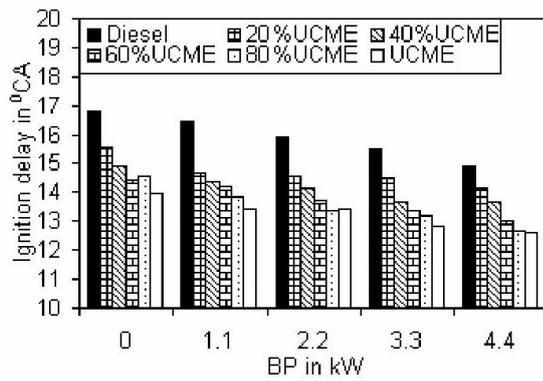
**Figure 2.** Comparison of ignition delay
