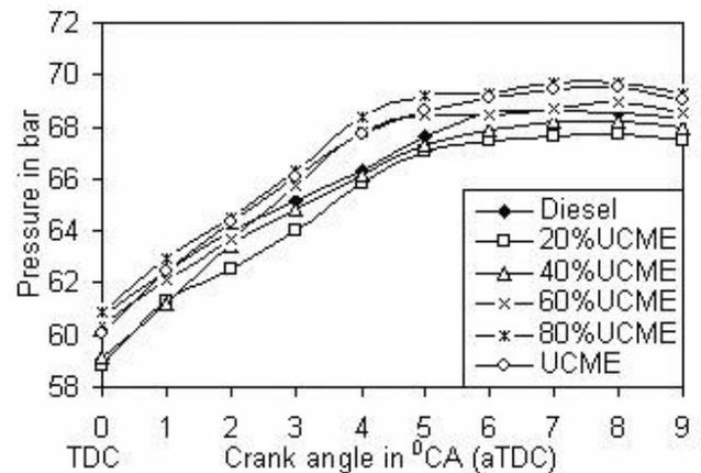
**Figure 5.** Comparison of In-cylinder pressure
