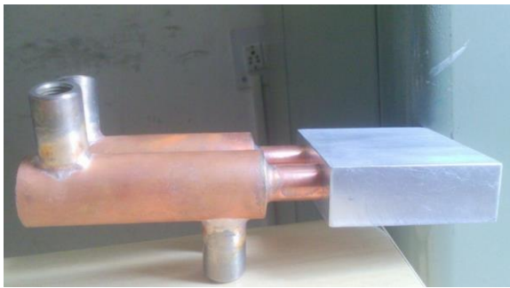
Figure3: Heat sink (Heat Pipe) with heat spreader
