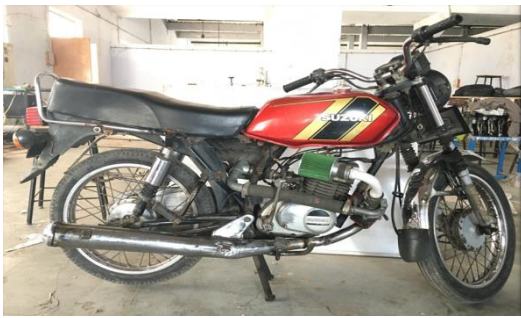
Figure 3. Installed Turbocharger system in 2-stroke bike.
