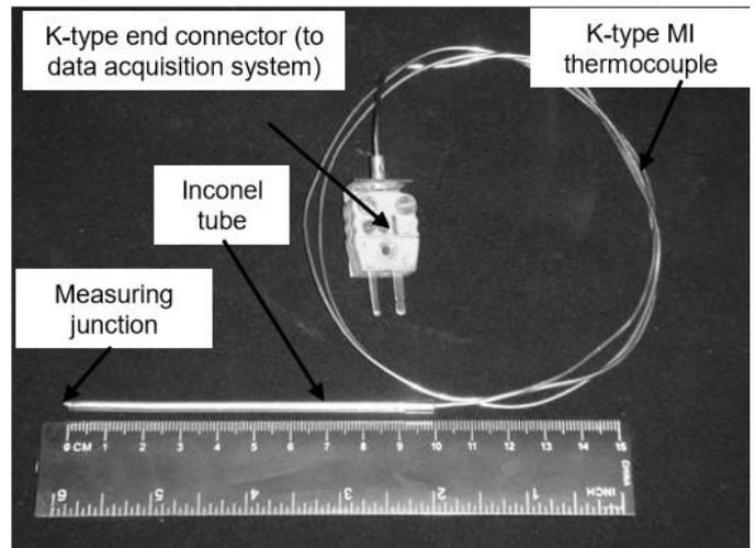
**Figure 6.** Typical K-type MI thermocouple assembly
