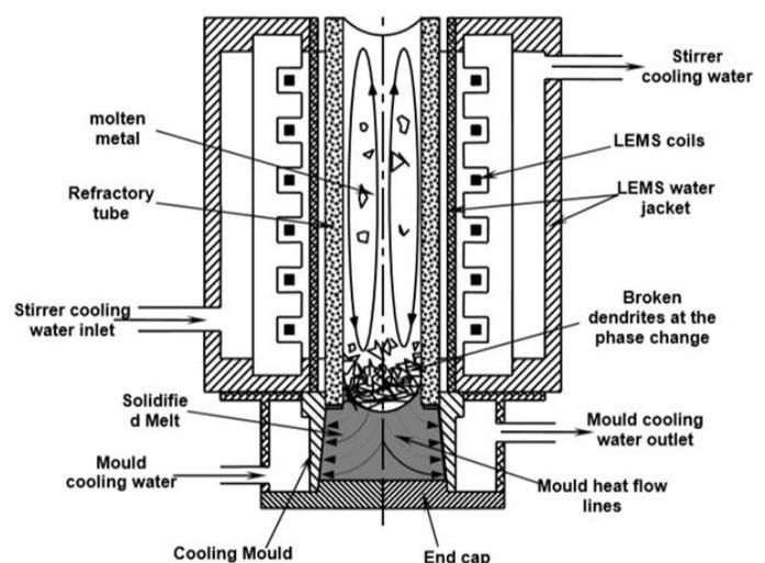
Figure 2. Schematic of rheocasting assembly
