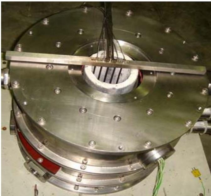
**Figure 7.** Melt temperature measurement with thermocouple “T” bar assembly
