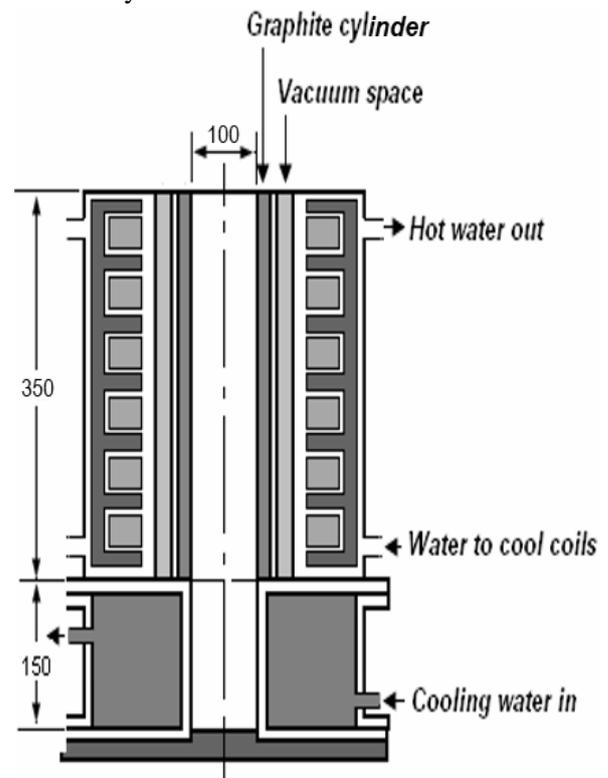
**Figure 1.** Schematic of rheocasting arrangement
