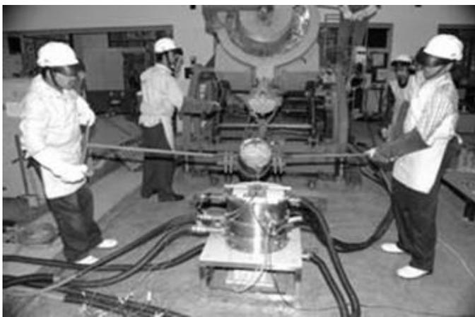
(b) Pouring into rheocast mould
