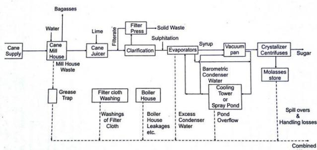
Figure 1: Flow Diagram for Sugar Manufacturing Process
