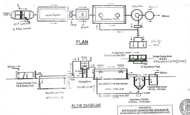
Figure 5: Process Flow Diagram of ETP of Industry.
