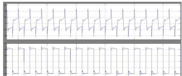
Fig 6: Output of BHB and FB Circuit
