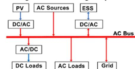
Fig 2: General AC grid system
