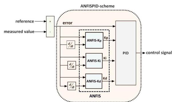
Fig 10: : General structure of ANFISPID-based control scheme
