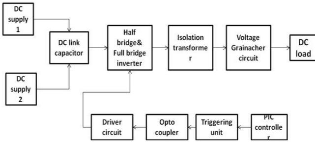
Fig 3: Block diagram of Proposed hybrid converter
