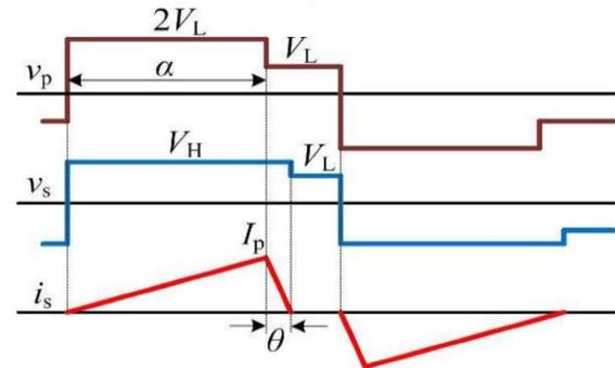
Fig 7: Typical waveforms under discontinuous  $I_s$
