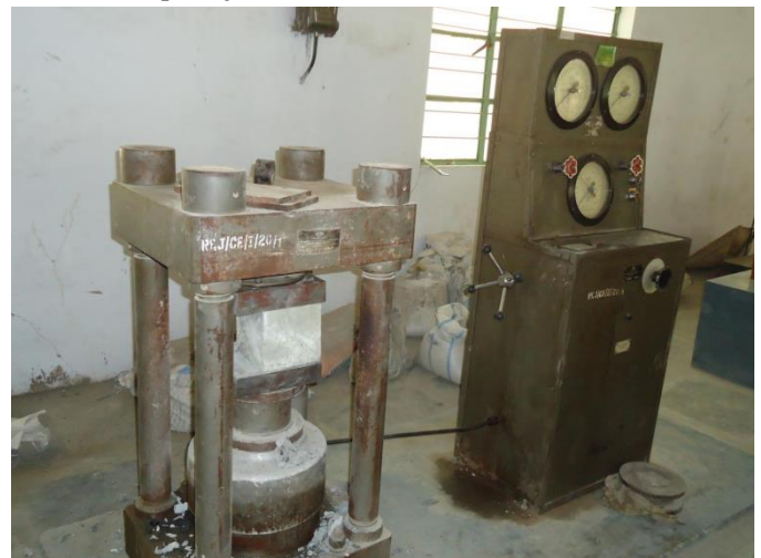
TESTING OF CUBES FOR DETERMINING COMPRESSIVE STRENGTH.
