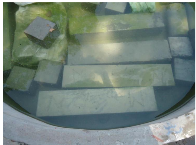
Curing of Beams, Cubes and Cylinders.
