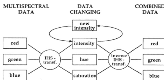
**Figure 2.** Principle of combination multisensor data
