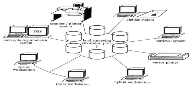
Figure 6. Decentralized hardware architecture including workstations
