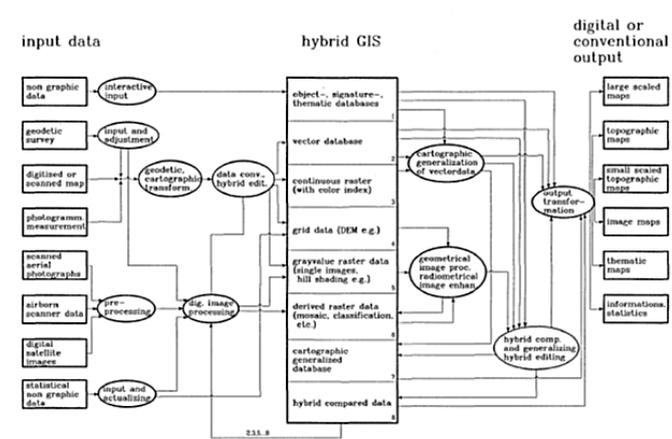
Figure 5. Hybrid GIS system architecture
