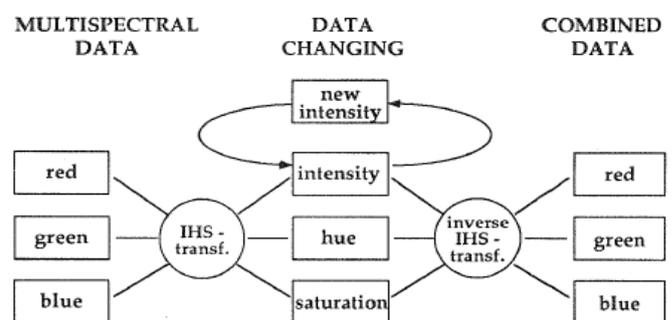
**Figure 2.** Principle of combination multisensor data
