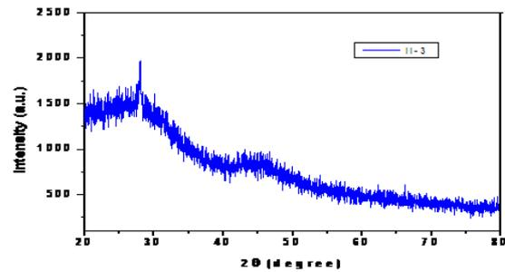
Figure 2. XRD profile for typical sample II-3 (X=25%).
