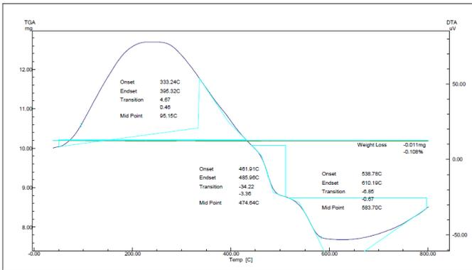
**Figure 5.** TGA-DTA curve and characteristic temperature determined for the Compositions  $x=15\%$  of  $P_2O_5$  glass at heating rate of  $40^\circ\text{C}/\text{min}$ .
