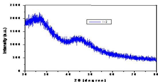
Figure 1. XRD profile for typical sample I-2 (X=20%).
