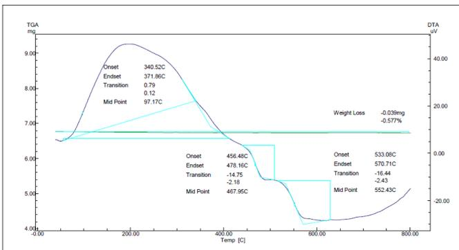
**Figure 6.** TGA-DTA curve and characteristic temperature determined for the Compositions  $x=25\%$  of  $P_2O_5$  glass at heating rate of  $40^\circ\text{C}/\text{min}$ .
