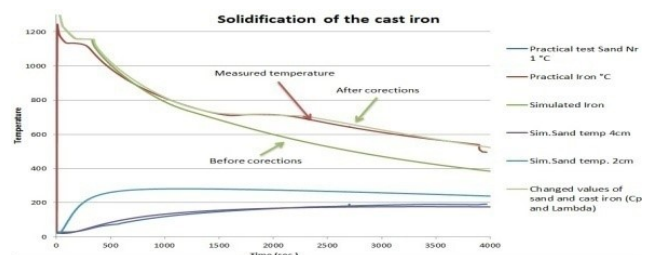
Figure 15. Calibration of the simulated solidification process of GJL-250.
