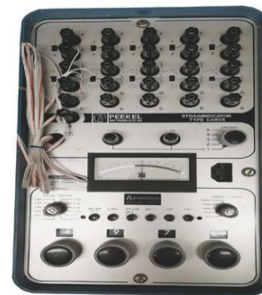
Figure 2. The tool used to measure the strain generated from the Wheatstone bridge to measure resistance in a strain gauge. Following is an example of how the stress is calculated from measurements:
