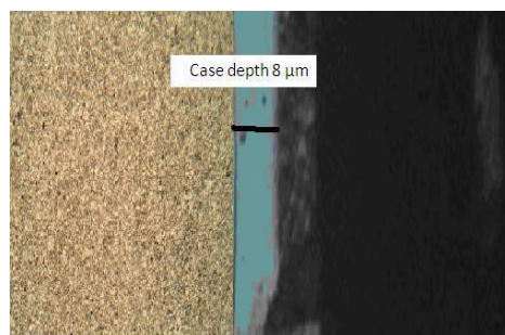
Figure 3. Induction hardening specimen for 1 minute
