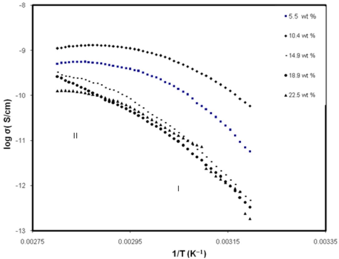
**Figure 2.** Variation of  $\log \sigma$  with  $1/T$  for different wt. % of Iodine
