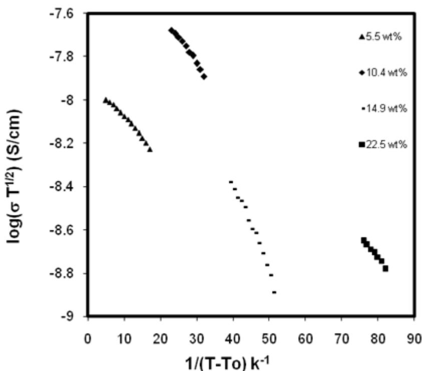
Figure 3. VTF plots for PTh-PVAc films for different wt % of Iodine
