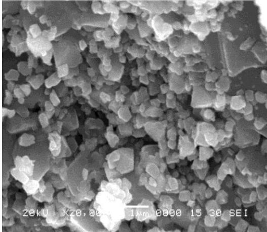
**Figure 4.** Typical SEM image of  $\text{CoCr}_x\text{Fe}_{2-x}\text{O}_4$  nanoferrite system
