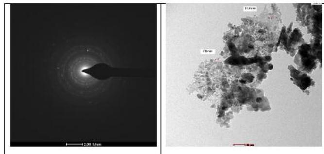
**Figure 3.** TEM micrograph of  $\text{SnO}_2\text{-ZnO}$  nano composite
