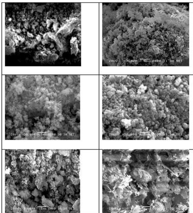
**Figure 2.** SEM micrograph of  $\text{SnO}_2\text{-ZnO}$  nano composite
