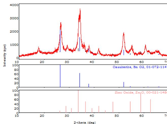
Figure 1. XRD pattern of SnO<sub>2</sub>-ZnO nano composite
