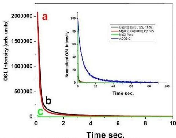
**Figure 2.** CW- OSL Response in NaCl (a) NaCl:Ca,Cu,P (b) NaCl:Mg,Cu,P (c) NaCl:Cu
