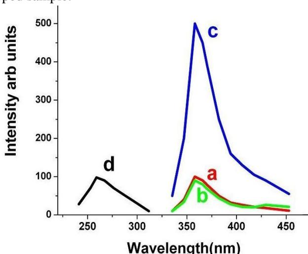
**Figure 1.** Photo-Luminescence in NaCl: Emission (a) NaCl:Ca,Cu,P (b) NaCl:Mg,Cu,P (c) NaCl:Cu Excitation: (d)For all samples of NaCl.
