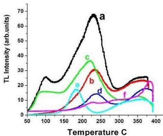
**Figure 3.** TL Response in NaCl (a) NaCl: Ca,Cu,P (b) NaCl: Mg,Cu,P (c) NaCl:Cu
