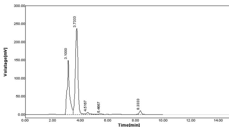
**Figure 29.** Chromatogram of stability for Acid Degradation (0.1 N HCl) ( After 1 Hr)
