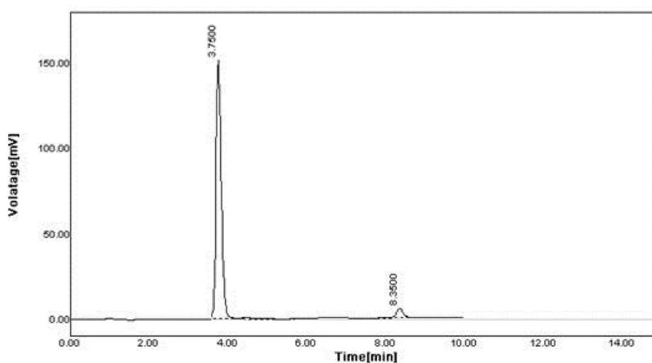
**Figure 23.** Chromatogram of Robustness Changing of mobile phase by (81-19)**Table 23.** Changing mobile phase by (79-21)
