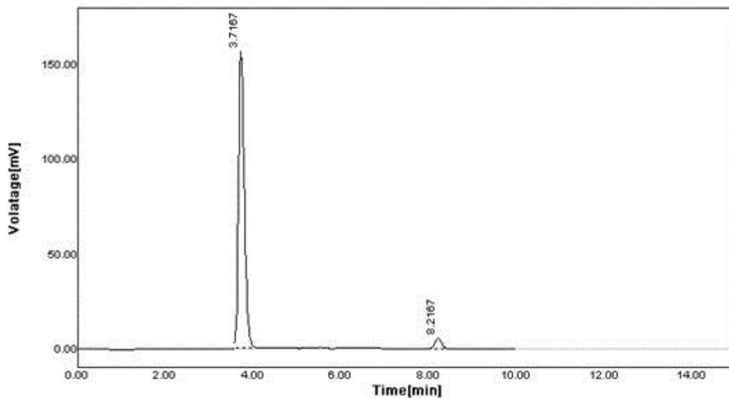
**Figure 27.** Chromatogram of Robustness Changing wavelength by +237 nm.
