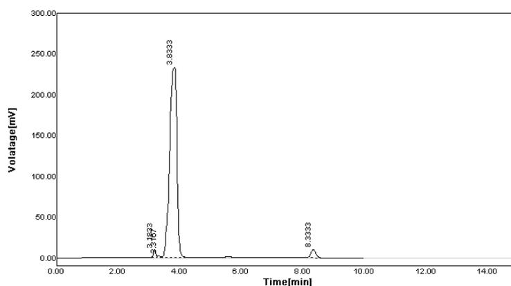
**Figure 30.** Chromatogram of stability for Base Degradation of 0.1N NaoH ( After 1 Hr)
