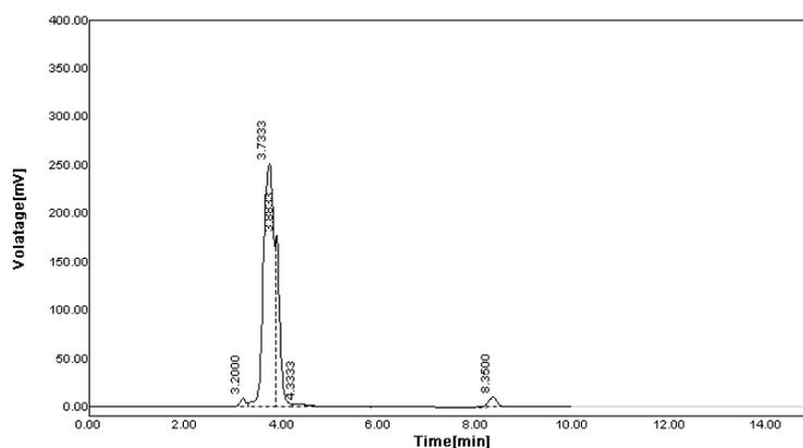
**Figure 33.** Chromatogram of stability for Base Degradation of 1N NaOH (After 1 Hr)
