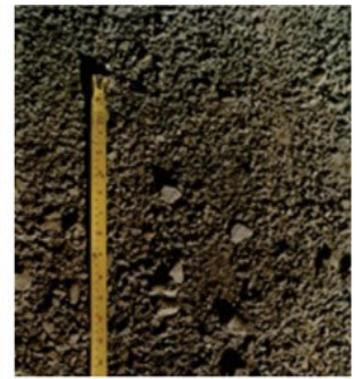
Jaw crushed sand-Flaky
