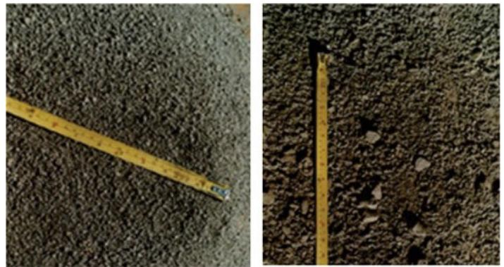
VSI Crushed Sand –Cubical      Jaw crushed sand-Flaky
