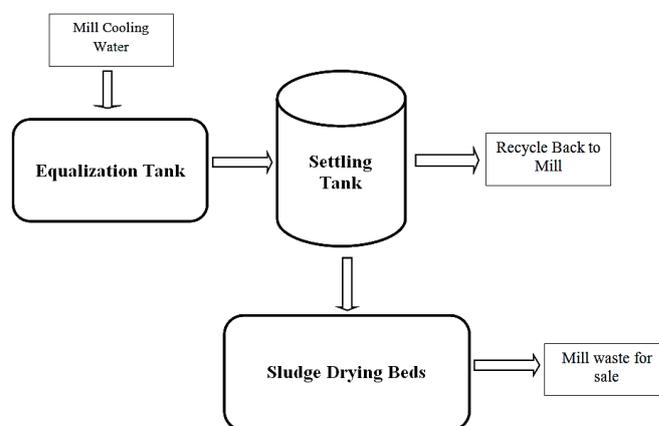
Figure 2 : Process Flow Diagram of ETP of Industry
