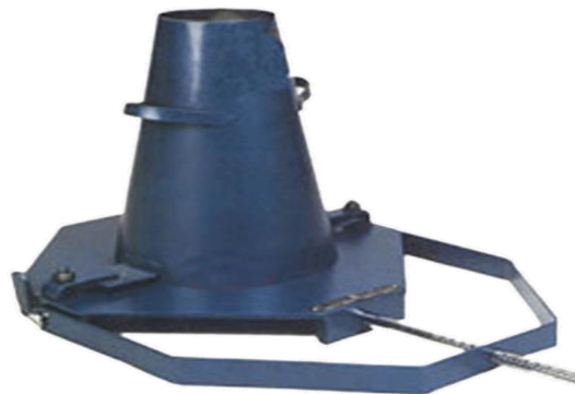
Slump cone test
