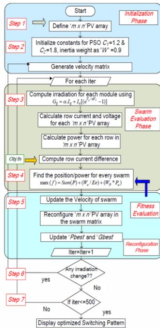
Figure 2. Flow Diagram
