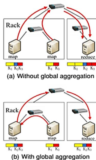
Fig. 2. Two schemes of intermediate data transmission in the shuffle phase.
