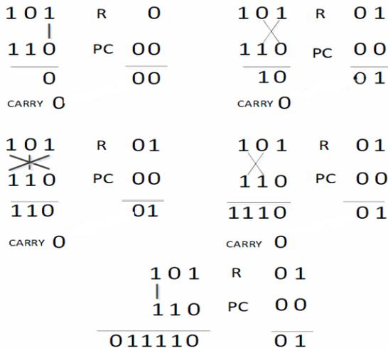
Figure 4 : Example of Urdhva Tiryakbhyam algorithm
