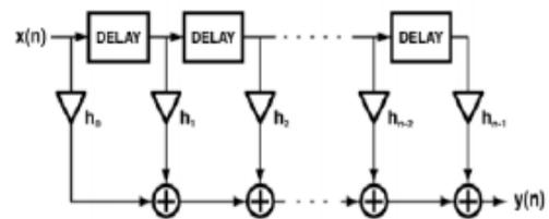
Figure 1: Transposed form FIR filter
