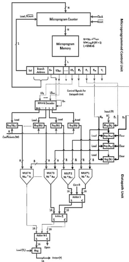
Figure 2 : Architecture of parallel microprogrammed FIR filter
