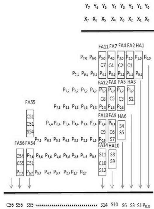
Figure 3 : Wallace tree multiplier using full adders and half adders
