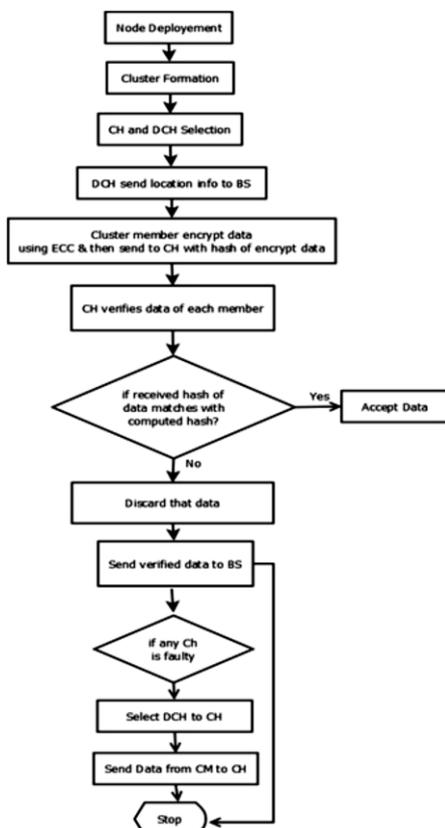
Figure 1. System Architecture
