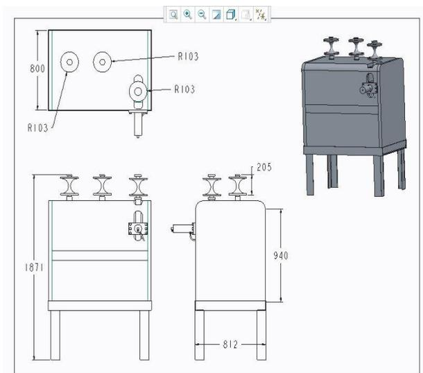
**Figure 1.** Sketch of single stage three roller pipe bending machine
