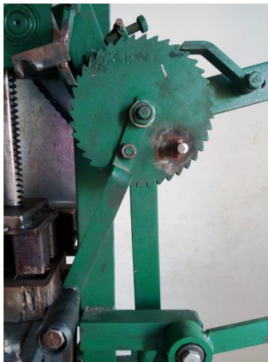
Figure 6. Actual diagram of Ratchet and Pawl
